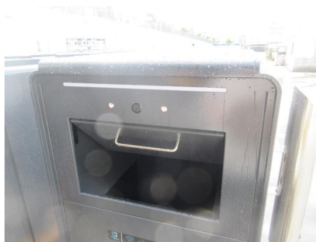
Automatic door and compactor can work normally after waterproof testing
