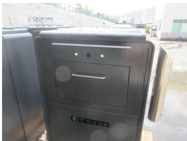
Automatic door and compactor can work normally after waterproof testing
