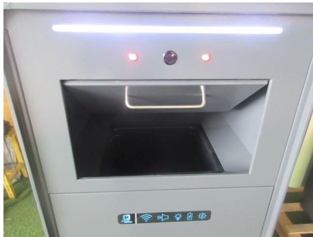
When the automatic door opens, green indicator light turns to red color.
